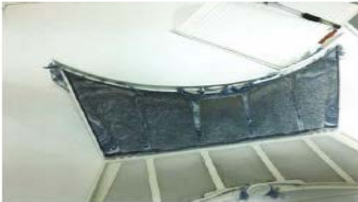
Totally blocked filter of a domestic type tumble dryer
